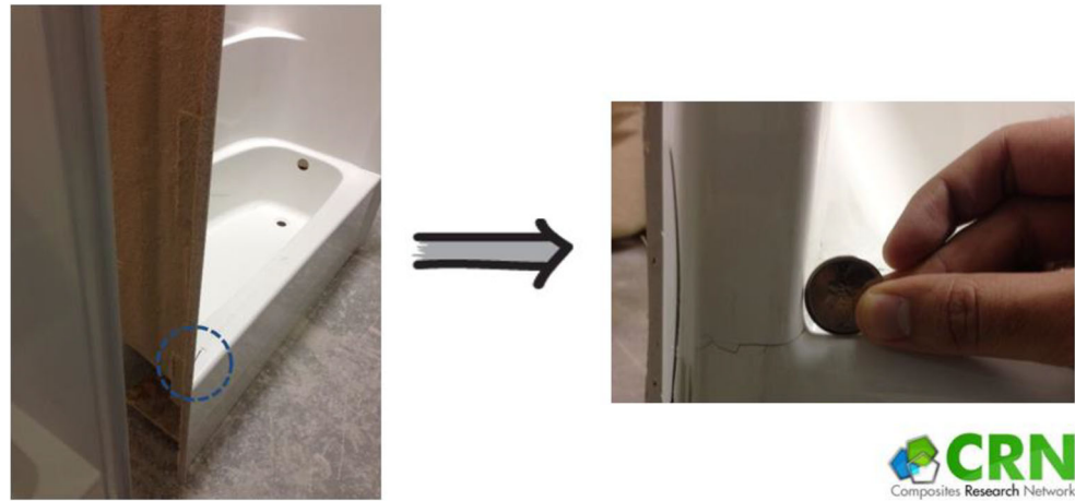
Fig. 3 Example of a corner crack defect, seen in tub showers after de-moulding
